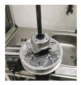
b. Lower the cam plate with the compression tool until the retaining ring appears.
