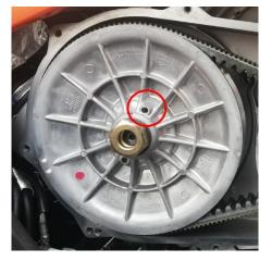
3. Remove driven pulley. Use 36 mm wrench to loosen the driven pulley nut.
