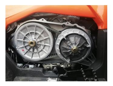
2. Loosen variator belt by screwing M6 bolt into the driven pulley at the locations shown in the picture.
