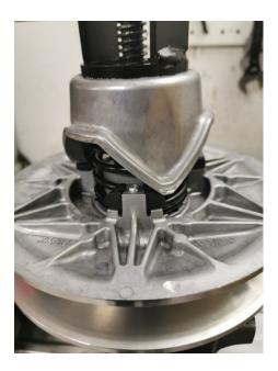
Spring zero position by example of position *C-1*
