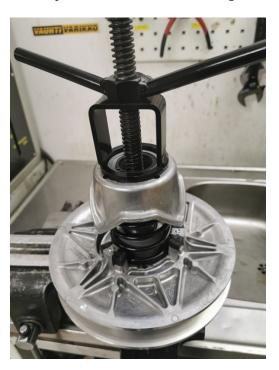
b. Turn the cam plate counterclockwise to pre-stress the spring according to the selected position and the angle indicated in Annex 1, page 10. Example: position C-1=34 degrees from the spring zero position so it means you have to turn the cam plate until the next cam shoe. Make sure that the cam plate goes to the right side of the cam shoes (see picture on point 5c).
