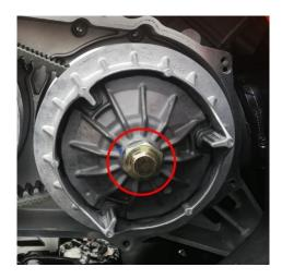
2. Remove the cover plate nut. Use 30 mm wrench. NB! Nut has left hand thread!
