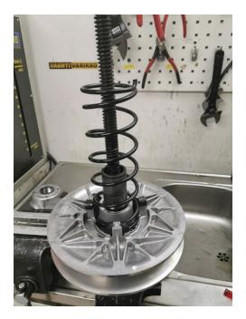
5. There are holes in the cam plate and sliding flange for position the spring. In the cam plate, the holes are marked with numbers (1,2,3,4) and in the sliding flange, the holes are marked with letters (A, B, C).
